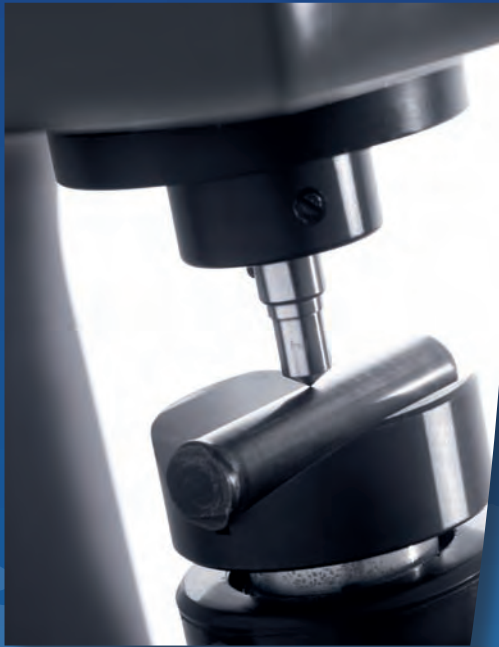
Pin hardness measuring
