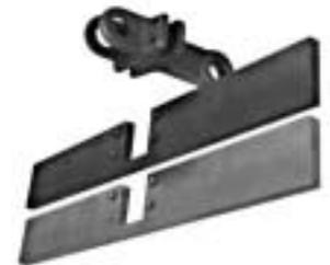
This chain type requires the use of non-symmetrical sprocket plates.
