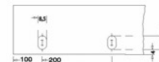
Holes on flange C-14 y C-15
