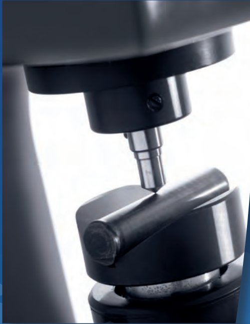
Pin hardness measuring
